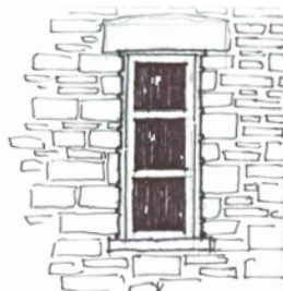
Windows with vertical proportions.
